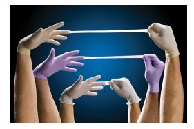
Three types of base glove materials (from top): natural rubber latex (NRL), acrylonitrile-butadiene (nitrile) and polyvinyl chloride (vinyl, PVC).
